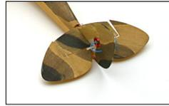
Join the elevator halves together with a 1/16 stick and attach the rudder and elevator to the tail surfaces with thin slivers of rubber band. Attach the actuator coils (I use rubber cement which is both strong and allows easy removal should it be necessary) and pass the wires through the small opening just behind rib F5. You may need to drill a small hole in the top of F5 to allow this.
