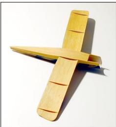
Once the ribs are in place, glue in the bottom wing and add the bottom sheet. You'll have to shave a small amount of wood from the center rear of the wing to allow the sheet to sit flat.
